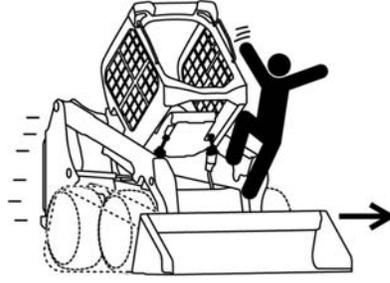
UN MOUVEMENT ACCIDENTEL DE L'ACCESSOIRE, DES BRAS DE LEVAGE OU DE LA CHARGEUSE PROVOQUÉ PAR UN CONTACT DES COMMANDES PAR LA CABINE PEUT ENTRÂINER DES BLESSURES GRAVES, VOIRE MORTELLES
